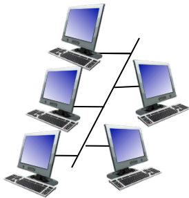
shared wire (e.g., cabled Ethernet)
